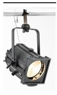
The Rama High Performance 175 FFT Fresnel (1.0kW / 1.2kW, 175mm lens) provides an adjustable cone of light has a soft edge and is easily blended with adjacent beams to provide even illumination. The large 175mm lens provides up to 50% more illumination than conventional 150mm Fresnels.
